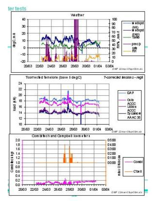
Fig. 4.8 Weather, conductor ice load and Icemeter data for late March, 2009. The Campbell/Rosemount shows good agreement but Combi-Tech barely indicates above noise level. No output from the HoloOptic
