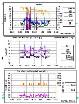
Fig. 4.6 Weather, conductor ice load and Icemeter data for early February, 2009. The Combi-Tech and Campbell/Rosemount show good agreement but no output from the HoloOptic
