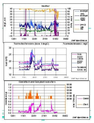
Fig. 4.5 Weather, conductor ice load and Icemeter data for late January, 2009. The Combi-Tech and Campbell/Rosemount show good agreement but no output from the HoloOptic
