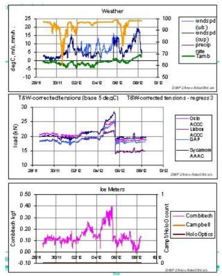
Fig. 4.2 Weather, conductor ice load and Icemeter data for early December, 2008. The Combi-Tech shows good agreement but no output from the other two icemeters.
