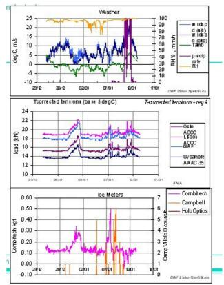
Fig. 4.4 Weather, conductor ice load and Icemeter data for early January, 2009. The Combi-Tech shows good agreement and the Campbell/Rosemount picks up the second incident but no output from the HoloOptic
