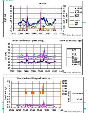
Fig. 4.7 Weather, conductor ice load and Icemeter data for early March, 2009. The Campbell/Rosemount shows good agreement but the Combi-Tech misses first two incidents and no output from the HoloOptic
